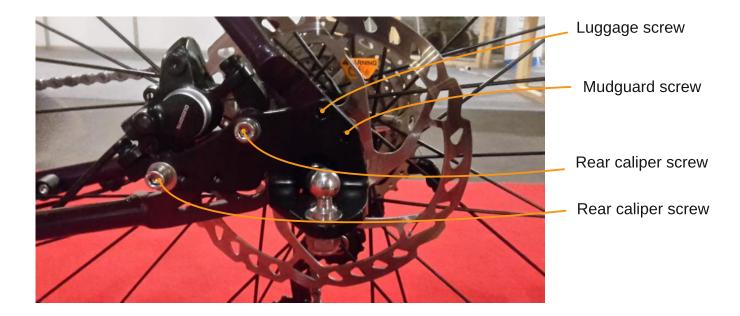
After assembly, check the rear brake of the bike for proper application and operation.
