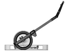
Check that the 2 sides are properly held by pressing on the front of the trailer: the rear of the load should lift symmetrically.
