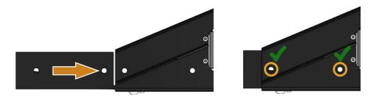
Fix the joint with the bolts, washers and M8 nuts supplied (5 mm Allen key and 13 mm open ended spanner).
