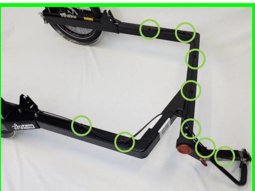
**Good condition of the cable housings which are fixed to the frame**
