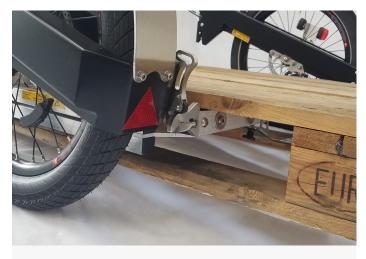
Integrated fixing points for easy lashing if necessary
