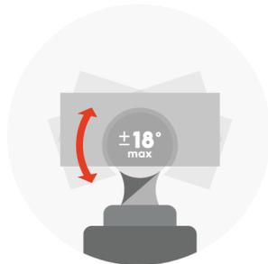
Limited front/rear angle around the hitch ball.
