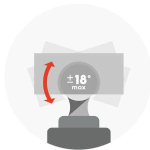
Limited front/rear angle around the hitch ball.
